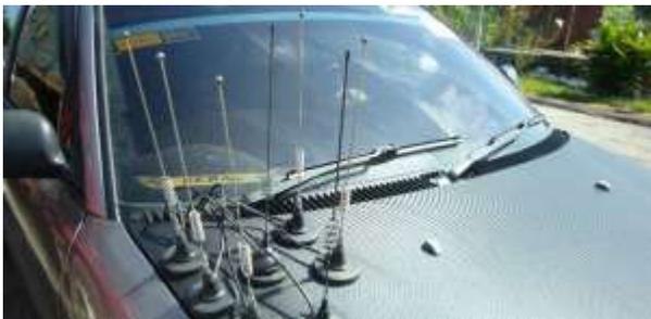
For auto/truck use, a mobile dual band antenna is the way to go. An HT connected to an outside antenna will work, but you will still need to be line of sight. As the terrain changes some power might be necessary. There are small amplifier modules that can connect to an HT. These can be located out of the way. Or you could consider a high power mobile/base unit.
