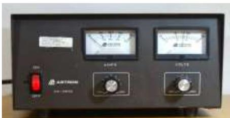
Any VHF/UHF mobile unit or HF radio when operated at home will require a 13.8 Volt DC power supply. There are two types of these, linear and switching. The linear is characterized by a larger size and heavier weight due to having a transformer inside. Until recently they were preferred because they do not radiate any noise and, therefore, don't cause any interference to our radio equipment. The switching
