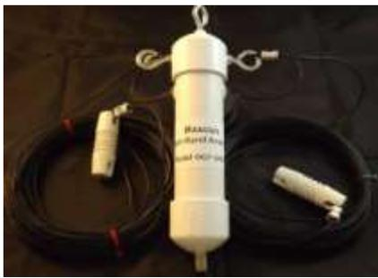
One offshoot of a dipole is the Off Center Fed dipole. This can give you multi-band performance with a single wire. These work very well and I have a couple of friends locally who use them. The lowest cost version is made by Maxcon antennas, their model OCF-3K80. Also needed is their in-line choke which keeps RF from getting onto the outside of the coax shield.
