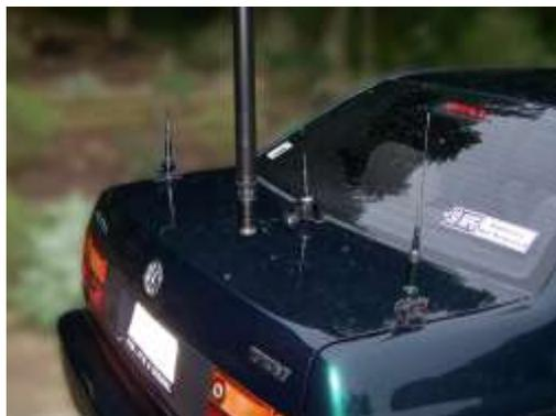
An antenna that is a  $\frac{1}{2}$  wave or full wave will not require any ground connection. A  $\frac{1}{4}$  wave (quarter wave) or  $\frac{5}{8}$ ths wave or  $\frac{3}{4}$  wave antenna will require some connection to the car body or some radiating wires at the base. Watch your garage clearance!
