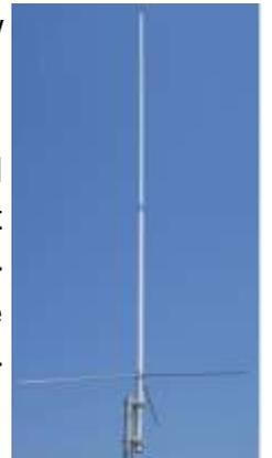
For FM repeaters only use a vertical antenna. Dual band, 144 + 440 MHz, are good choices. At home these can be clamped to any pipe. That includes the plumbing vent pipes we all have. If there is no alternative, put an antenna in an attic. All stock HT antennas are lossy. However, an HT connected to a proper antenna, perhaps with some gain, will show a marked and dramatic improvement. There are plenty of commercial dual band antennas available that aren't expensive.
