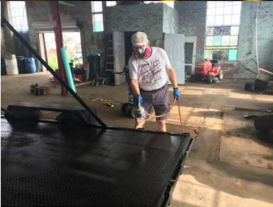
The Club's Antenna Trailer got a new steel floor. Over 3 days, the trailer floor was then sanded, cleaned, painted 2 coats, bottom sandblasted, & painted.
