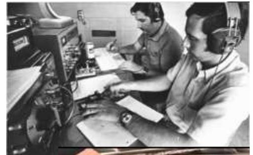
The HRO-60 receiver utilizes plug-in band coils.
