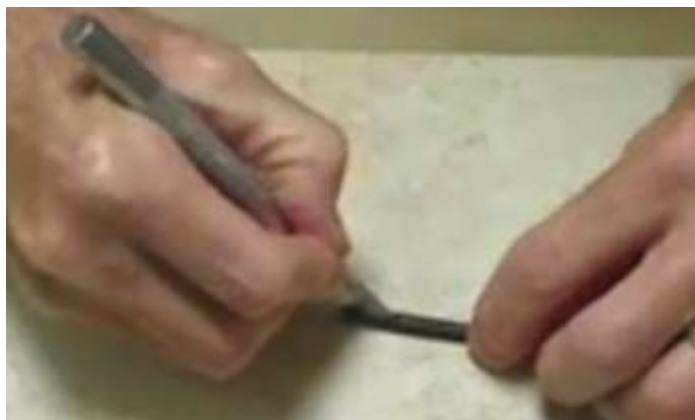
Cut to expose the inner cable
