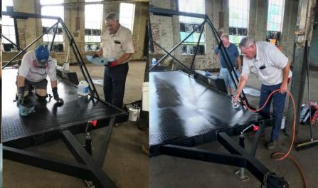
The Club's Antenna Trailer got a new steel floor. Over 3 days, the trailer floor was then sanded, cleaned, painted 2 coats, bottom sandblasted, & painted.
